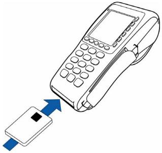
Figure 27 Inserting a Smart Card
